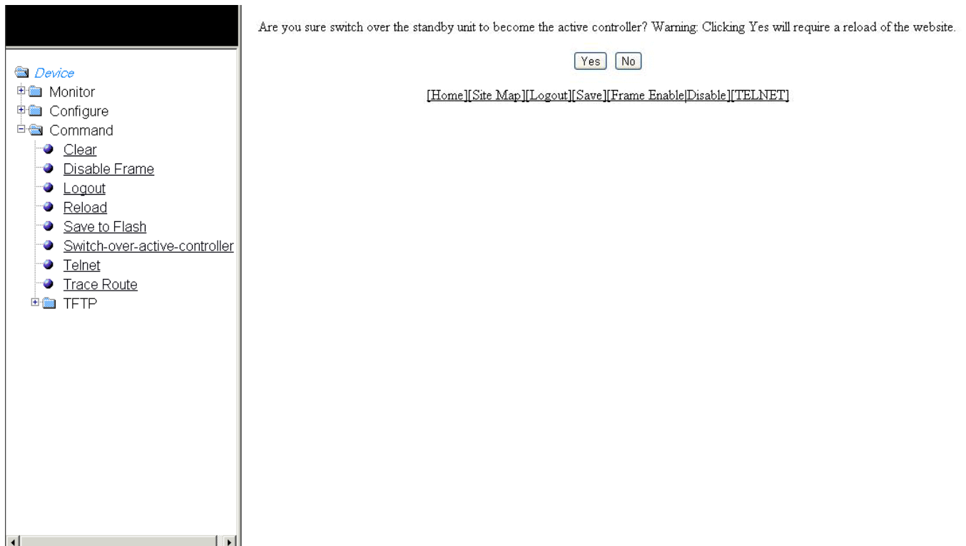
FIGURE 131 Switching over to an Active Controller
